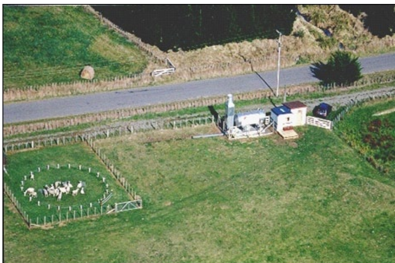
Figure 4.2. Aerial view of a single ring in the NZFACE also showing the bulk tank used to store liquid CO 2 .
